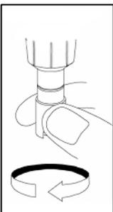
5. Thread the membrane cap onto the sensor. It is normal for a small amount of electrolyte to overflow.
