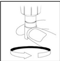
1. Remove the sensor guard or cal cup to access the sensor tip.
