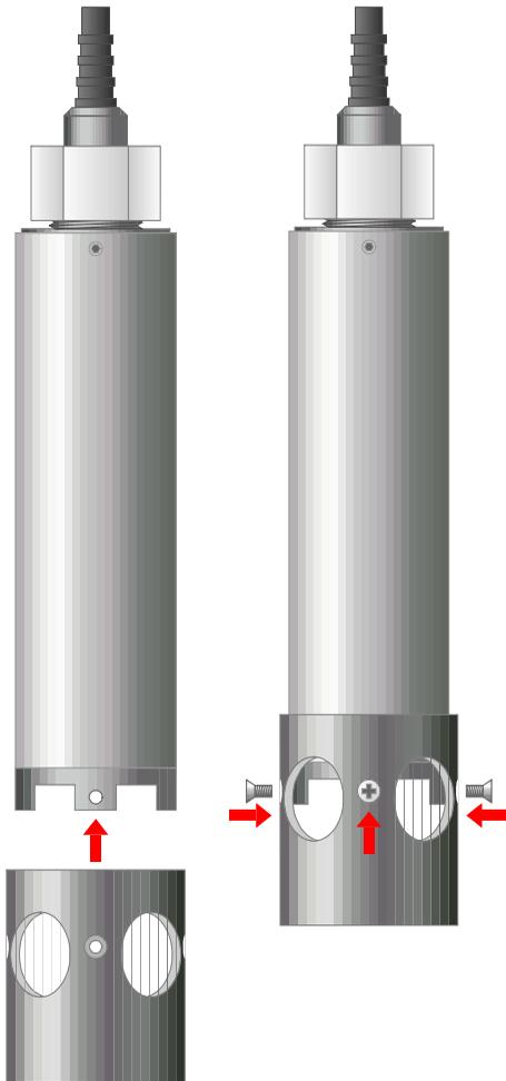
1. Slide the protector onto the Turbidity Sensor until the countersunk holes line up with the tapped holes in the sensor's four feet.
