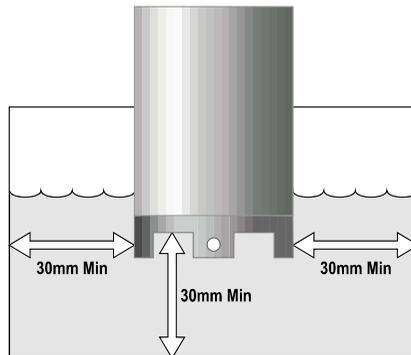
Take care to ensure that there are no bubbles trapped on the underside of the sensor. Bubbles can interfere with Turbidity measurements. Gently stir the sample or the sensor to dislodge any bubbles.
