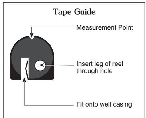
**Note:** When using the Tape Guide, the measuring point is offset from the top of casing. To adjust your measurements to the top of the casing, subtract the amount indicated on the front of the Tape Guide (i.e. 6 cm or 2/10 ft).
