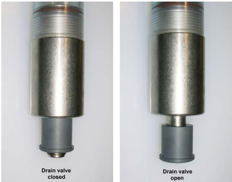
Figure 2-1 Drain valve operation
