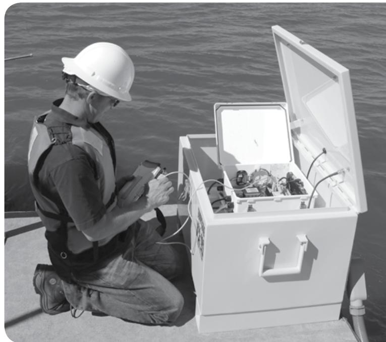
**An example of a NEMA enclosure where PLC + Modbus adapter are wired.**
