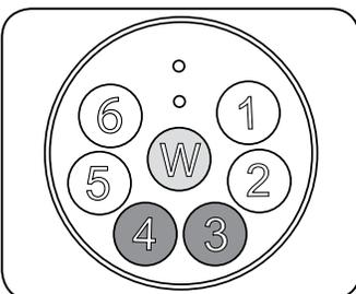
**EXO2 Optimal Wiped C/T positions: 3 or 4**
