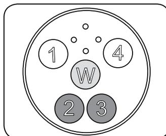
**EXO3 Optimal Wiped C/T positions: 2 or 3**
