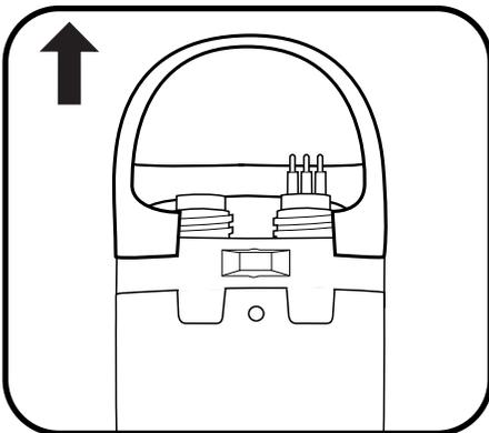
Once screws are removed, lift the bail off the sonde.
