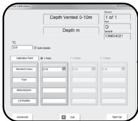
In the desktop KorEXO Calibrate menu, select Port D-Depth, then select Depth m from the second menu. In the Device Calibration menu, you should see Depth Vented 0-10m as the device name. (In the handheld KorEXO Calibrate menu, select Port D Dep V 0-10m, then select Depth m from the next menu.)
