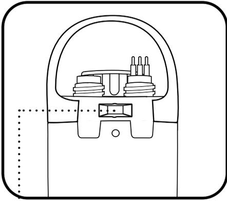
Indentation for location or positioning pin to ensure consistent horizontal orientation
