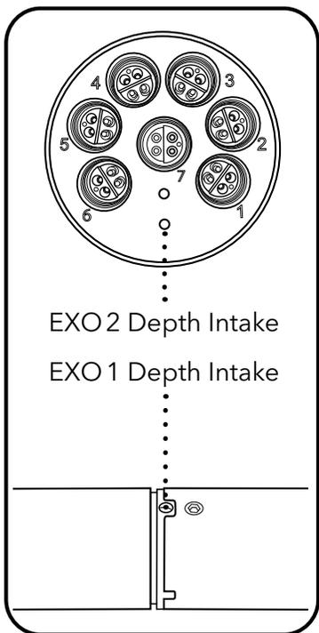
The sonde should be installed with at least 1 cm of water above the intake ports. If a conductivity sensor is installed, the depth will be compensated automatically for changes in the density of water as temperature and salinity change.
