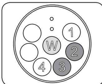
**EXO2 Optimal Wiped C/T positions: 2 or 3**
