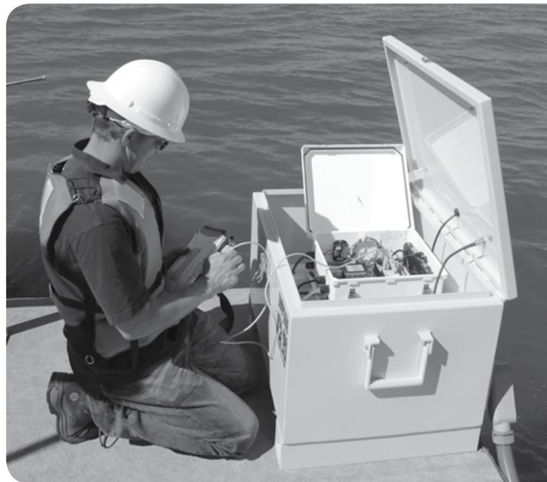
**An example of a NEMA enclosure where PLC + Modbus adapter are wired.**
