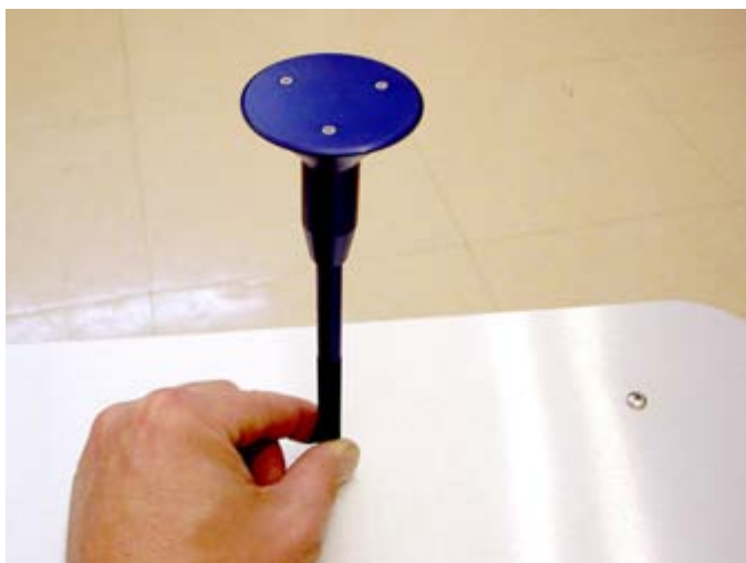
Figure 7: Thread the Inlet into the Inlet Ring after Heat Shield is Installed
