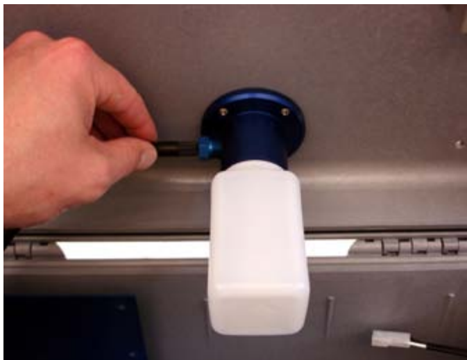
Figure 9: Install the Barbed Inlet Fitting and Sample Inlet Tubing
