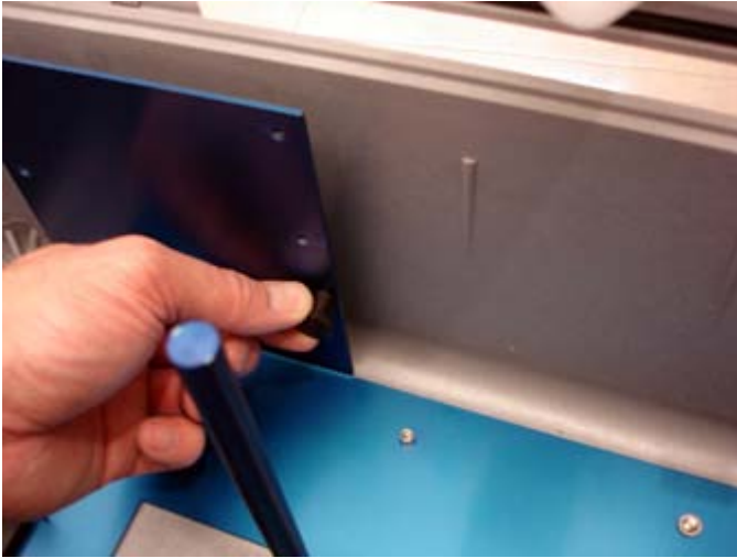
Figure 12: Store the Antenna Cable Fitting Plug
