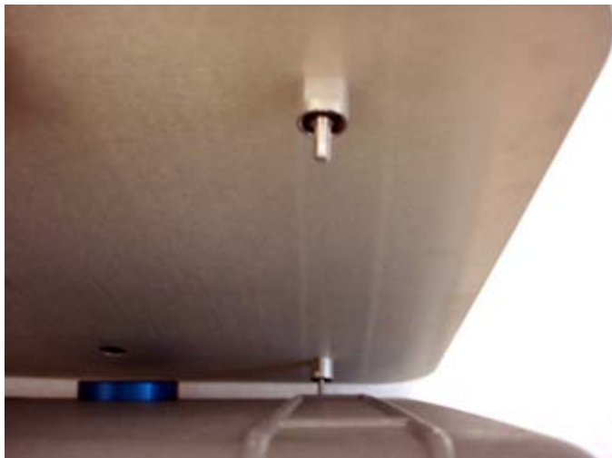
Figure 6: Attach Heat Shield to the top of the Enclosure
