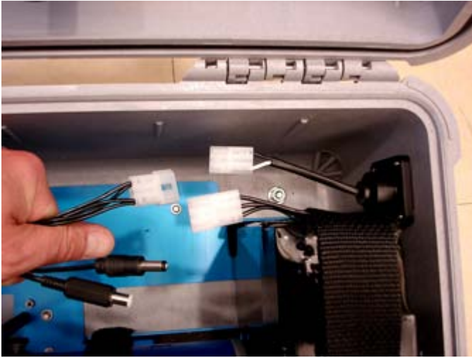
Figure 30: Internal DC Power Connections
