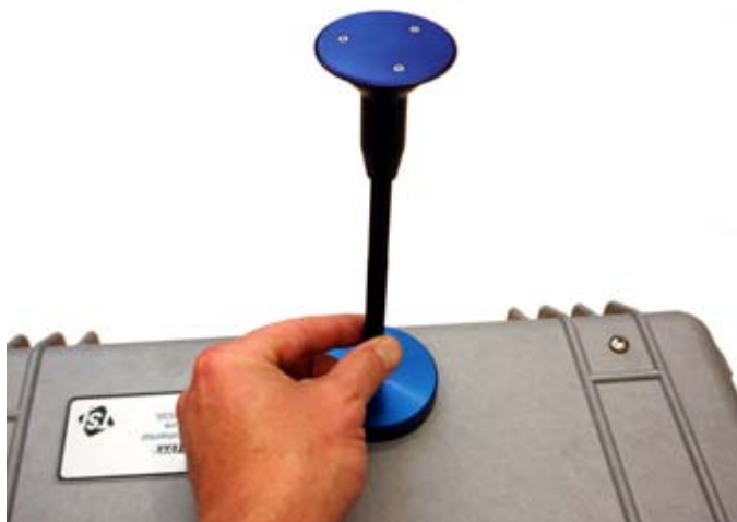
Figure 4: Thread the Inlet into the Inlet Ring
