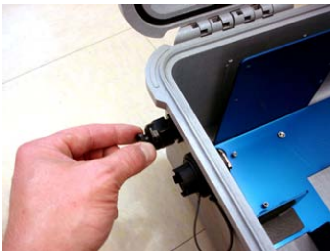
Figure 11: Remove the Antenna Cable Fitting Plug
