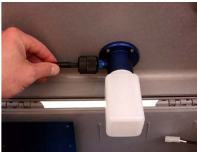
Figure 10: Install Impactor in the Sample Flow
