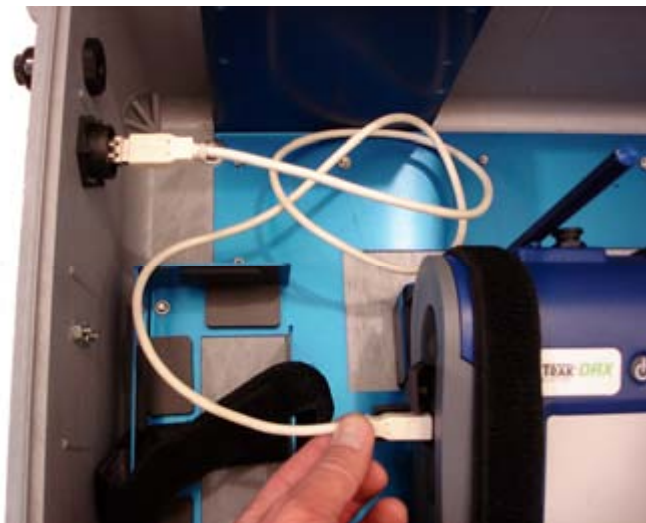
Figure 28: Connect USB Cable for Pass-through
