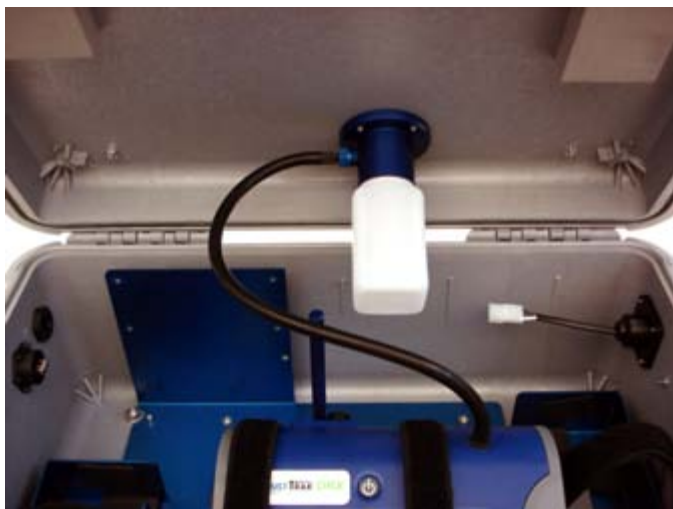
Figure 29: Connect Sample Tubing
