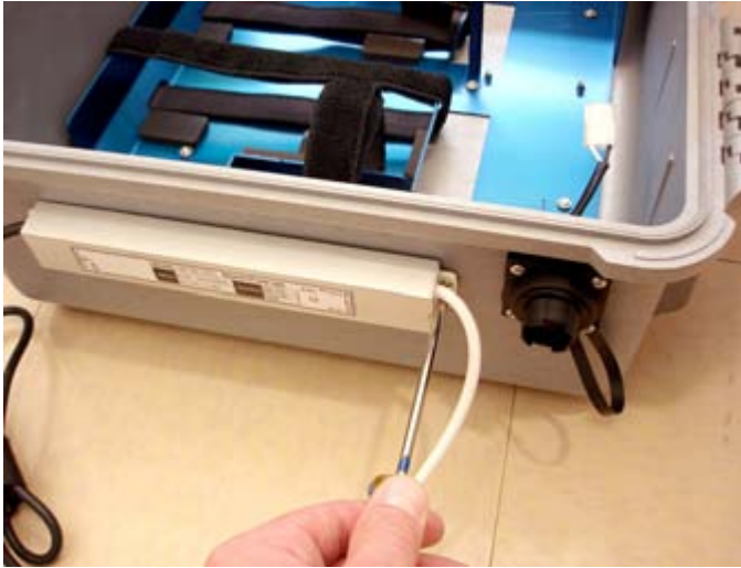
Figure 23: Attach the Adapter to the Enclosure
