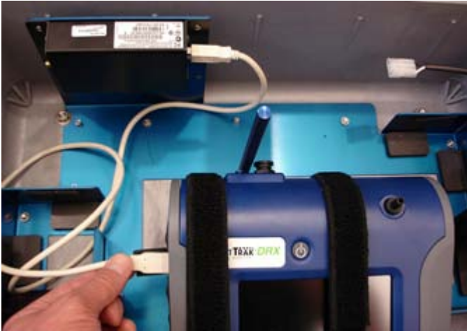
Figure 27: Connect USB Cable for Radio Modem
