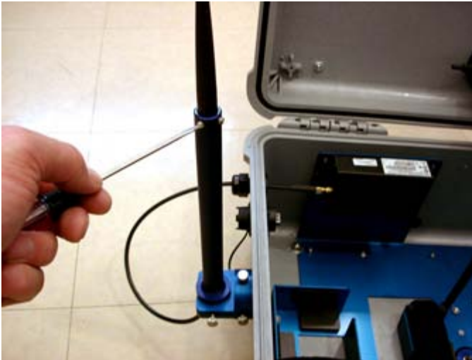
Figure 17: Secure Antenna to Bracket
