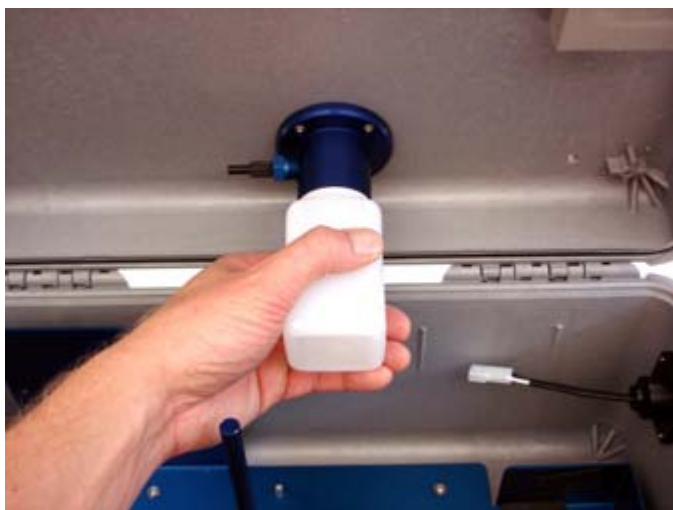
Figure 8: Install the Water Trap Bottle
