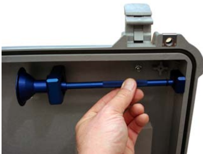
Figure 3: Unscrew Inlet from Inner Bracket
