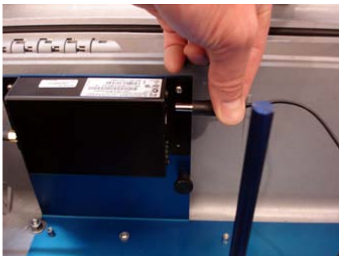
Figure 19: Power Connection to Radio Modem
