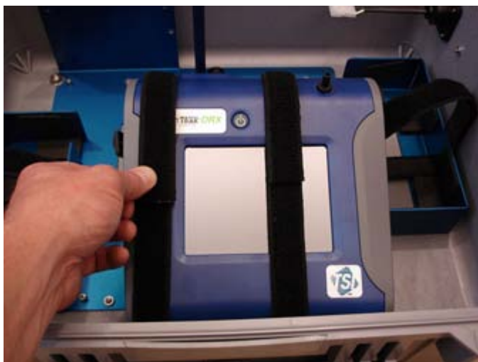
Figure 26: Install DUSTTRAK™ Monitor in the Bracket
