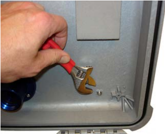
Figure 5: Remove Waterproof Bolt Assemblies from Heat Shield Mount Locations
