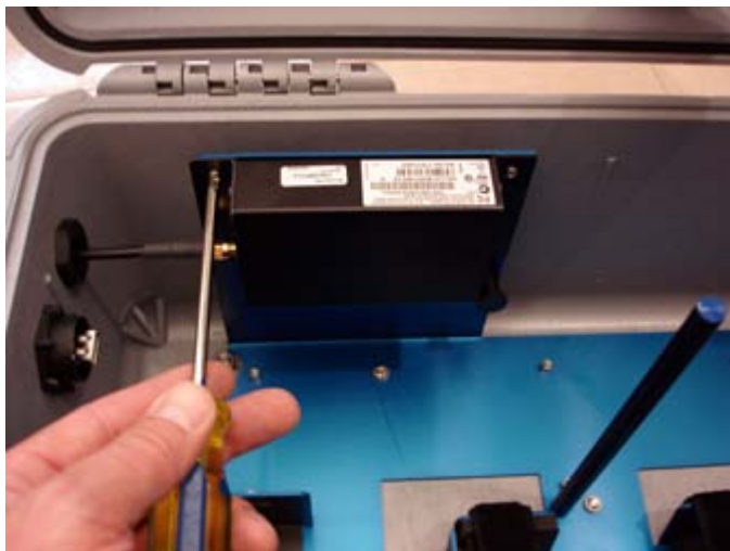
Figure 14: Attach Radio Modem to Bracket
