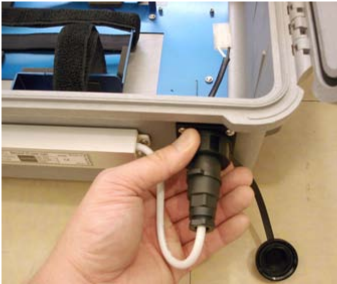
Figure 24: Connect Adapter DC Cable to Enclosure
