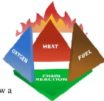
This is called the fire tetrahedron (formerly known as the fire triangle). If any of the four elements are missing, combustion cannot occur. The fourth element, chain reaction, means that not any mixture of fuel and oxygen can sustain a flame if heated. The proportions must allow a flame to propagate. For normal air, this means that the fuel concentration must be between the LEL and the UEL.
