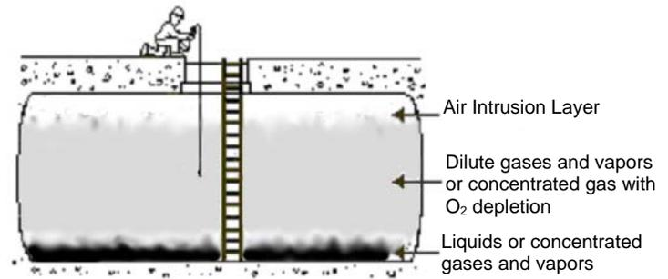
Before entering the confined space, take samples at several levels, and after entering, monitor the space continuously because conditions can change.
