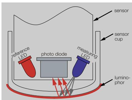
The excited luminophor radiates red light back with a time delay in a more or less short period of time (depending on the oxygen concentration). The classically determined decay time is a measure of the oxygen concentration. With a red LED, the sensor electronics undergoes a continuous “null” adjustment.
