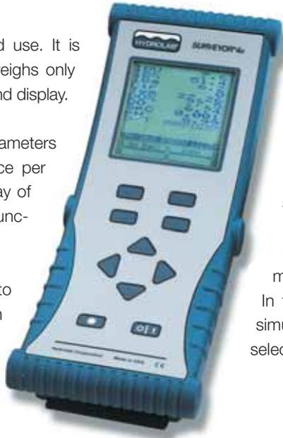
The Surveyor can provide power to the probes as it is performing the measurements, with the average power duration being 12 hours depending on the configuration selected.
