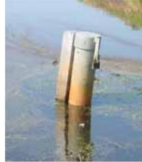
If a steel pipe is used (see pictures) with a 1" monitoring well installed inside the pipe, allow the Diver's extremity to protrude somewhat beyond the end of the pipe so that the Diver's sensors also come into contact with the water at this point.
