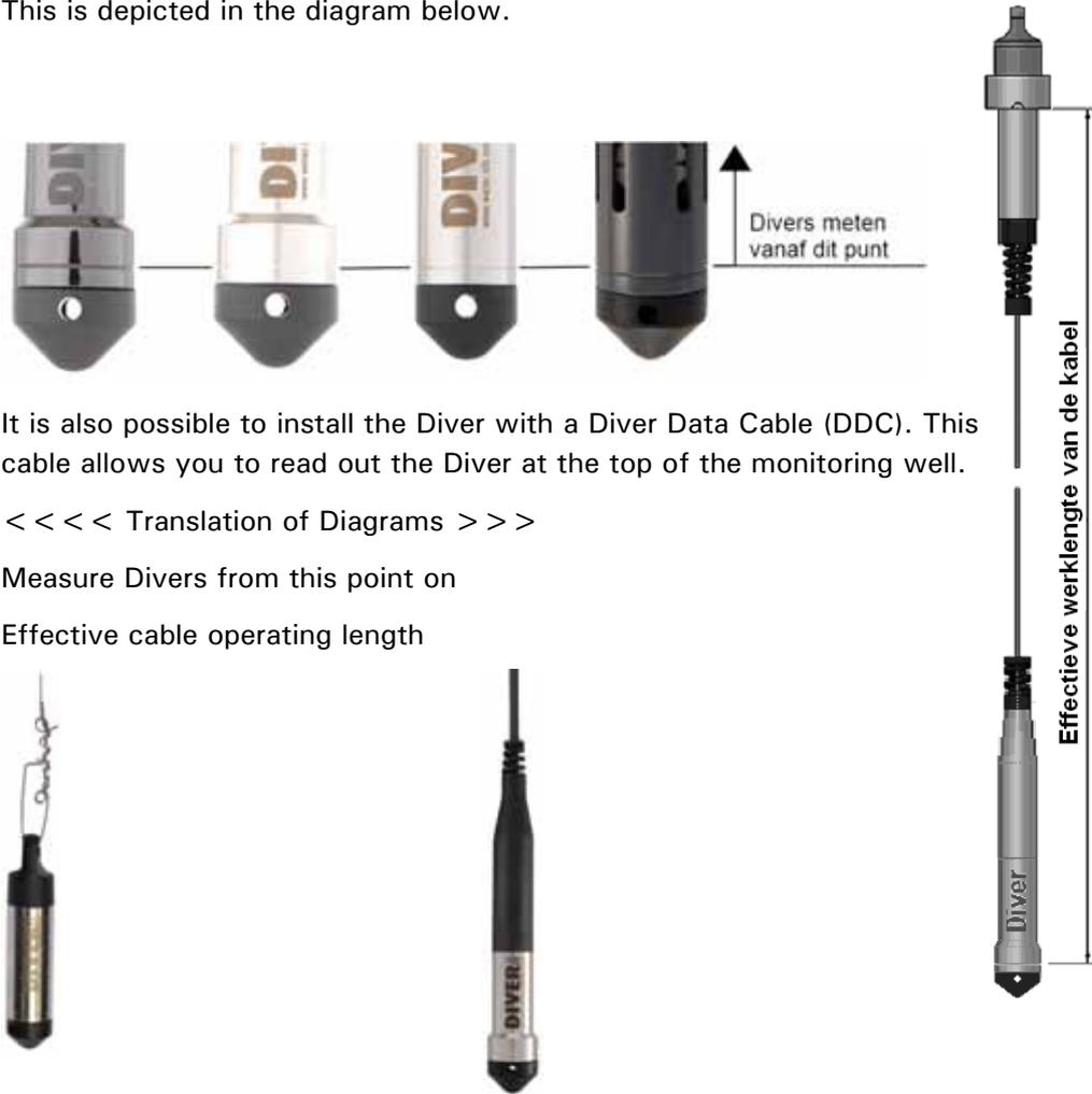
It is also possible to install the Diver with a Diver Data Cable (DDC). This cable allows you to read out the Diver at the top of the monitoring well.
